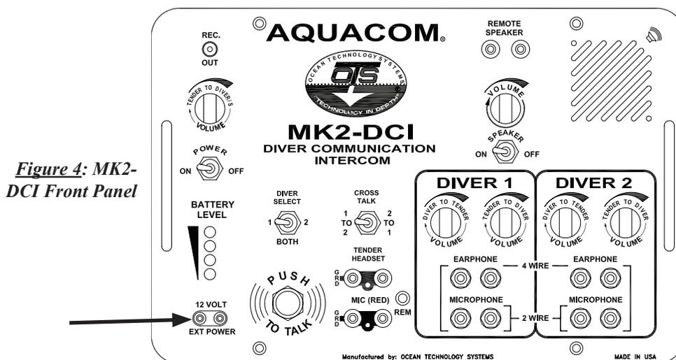
**Figure 4:** MK2-DCI Front Panel
