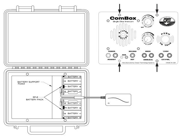
Figure 2: ComBox with cover removed and charger connected
