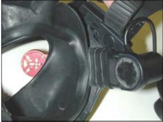
3. Install the microphone into the port. (The microphone will appear to be too large, but the seal easily stretches.) Pull the microphone and port into place.
