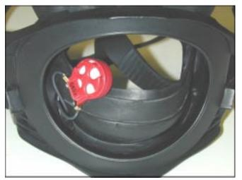
7. Don the mask and assure the microphone is positioned as close to your lips as possible, at the right corner of your mouth (less than 1/4 inch is best). The correct microphone position is important: If it is too far from your lips, communications will sound weak and distant.
