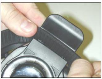
5. Fully insert the upper right head strap of the mask into the strap retainer slot on the M-48 Buddy Phone® so that the Buddy Phone® will be positioned over the right ear.
