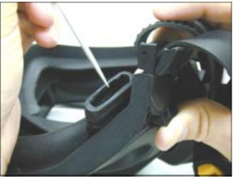
2. Using a sharp Exacto<sup>®</sup>-type knife, *very carefully* cut away and remove the center portion of the right microphone port.
