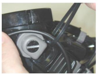
7. Install a tie wrap to secure loosely the Buddy Phone® cable to the upper prong of the upper left mask strap buckle (where the buckle attaches to the buckle holder on the mask). Cut off any extra length of tie wrap.
