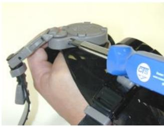
1. Remove the screw that secures the clamp on the diver's left accessory port of the mask. Set the screw and nut aside.
