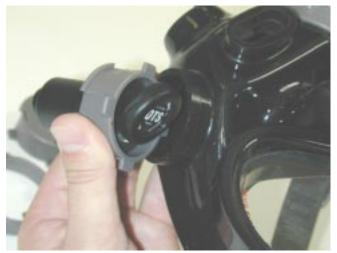
3. Insert the microphone/push-to-talk (PTT) module of the Buddy Phone® fully into the open accessory port so that the module rests evenly along the opening. Match the orientation of the opposite port's cap. The microphone should be positioned at a 45-degree angle relative to the front inner surface of the mask.
