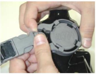
2. Open the clamp that attaches the mask strap, releasing the tabs that hold the cap onto the accessory port. Remove the cap from the port.
