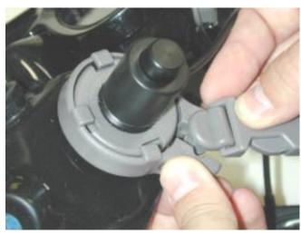
4. Install the clamp onto the PTT assembly cap, ensuring the strap buckle is attached to the clamp. Close the clamp's tabs onto the cap so that the assembly is fastened securely.
