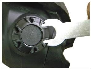
1. Locate the communications port on the right side of the mask. Using the OTS wrench¹ (p/n 137053-000; standard issue with Guardian FFM), unscrew the fastening nut from the plug counterclockwise and remove. The plug is then easily taken out from the inside of the mask.
