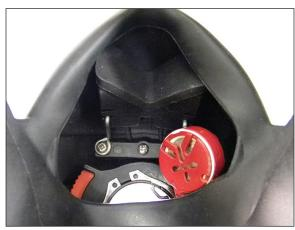
6. Once the microphone is inside the port, carefully position it within 1/4" of the right corner of the diver's lips. The ME-16R Hot-Mic® is shown above; other microphones are available (e.g., the Super Mic®, our patented\* all-depth, noise-cancelling microphone).
