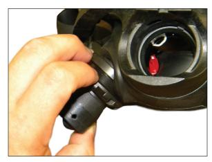
4. Continue inserting the microphone/PTT module into the communications port. The lip of the mask should go over the base of the module and rest between the base and the fastening nut.
