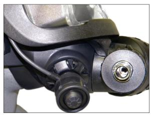
5. The fastening nut is then screwed down clockwise with the OTS wrench until tight against the mask. The OTS-BUD cable should be pointing towards the Buddy Phone® above the right ear.
