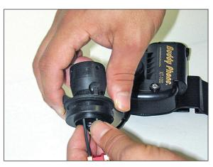
2. Loosen the captive fastening nut on the microphone/push-to-talk (PTT) module of the OTS-BUD counterclockwise so that there is space between the fastening nut and the base of the module.
