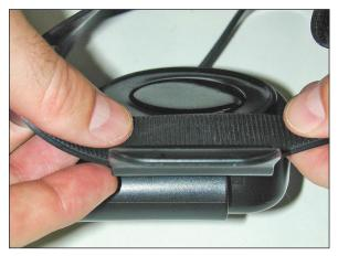
7. Fully insert the upper right head strap of the mask into the strap retainer slot on the OTS-BUD so that the Buddy Phone will be positioned above the right ear. Stretching the strap will make it easier to slip into the slot.
