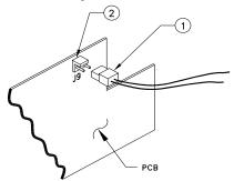
Figure 3. Battery Wire Harness Connection
