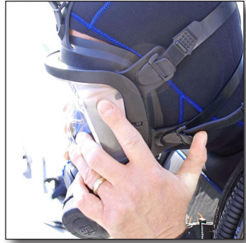
Figure 15: To Remove Mask, Use Thumbs to Grasp Bottom Buckle Tabs and Loosen
