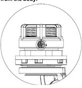
3: Remove check valve from the inner frame and replace with a new valve by pulling the small tab through the valve seat with a pair of needle nose pliers.
